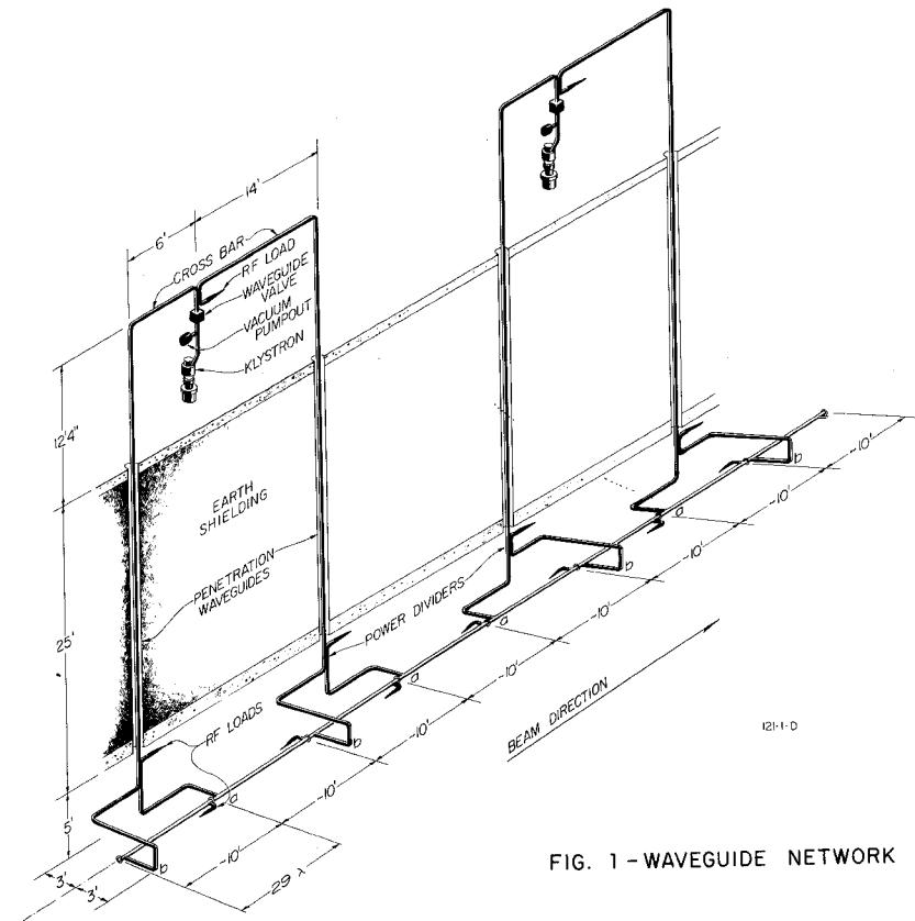
FIG. 1 - WAVEGUIDE NETWORK
